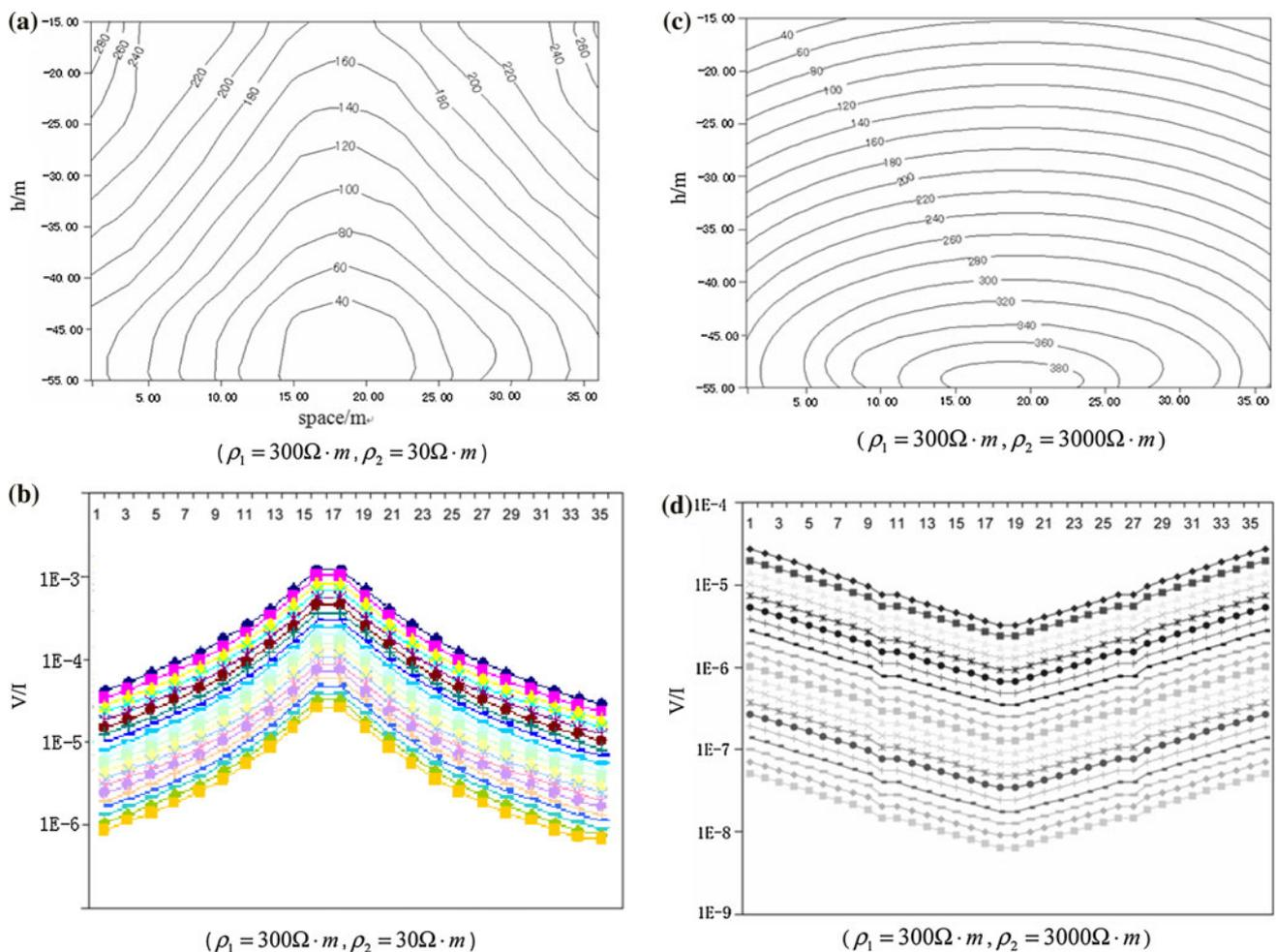
**Fig. 2** Apparent resistivity contour of 3-D resistance cave at 50 m depth from calculated result of conductive and resistance models. **a** Apparent resistivity contour of conductive body. **b** Multi-channel
