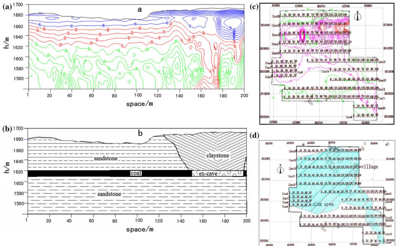
**Fig. 4** Apparent resistivity distributing and detected geological status. **a** Geodesic variation of the apparent resistivity at deep direction. **b** Geological structure status at deep direction obtained by
