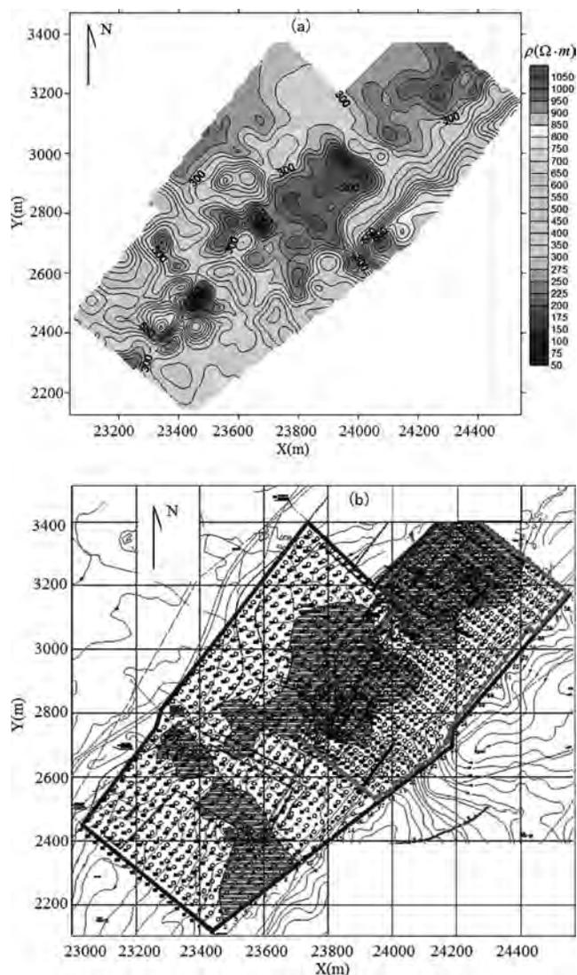
**Figure 9. Plan views of apparent resistivity contour and interpreted result. a) Apparent resistivity contour map. b) Interpreted anomaly areas shown in black.**
