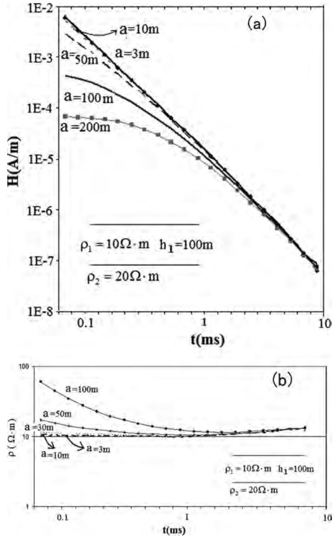
Figure 1. Model responses for the same magnetic moment ( $9,000 \text{ m}^2\cdot\text{A}$ ), but different loop radii ( $a = 200$  m,  $100$  m,  $50$  m,  $10$  m, and  $3$  m). a) Magnetic field decay curves; b) apparent resistivity curves.
