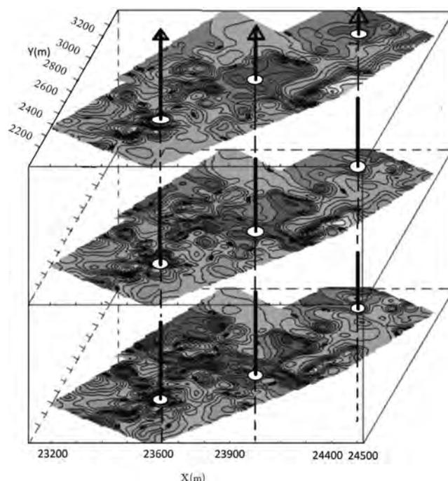
**Figure 10. Apparent resistivity contour depth slices at -150 m, -250 m, and -350 m and borehole locations.**
