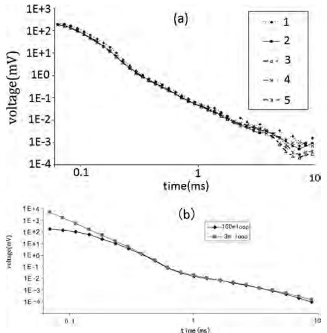
Figure 7. Testing and comparison survey using the EMRS-3 system. (a) Decay curves collected at the same location multiple times, showing the repeatability of the system. (b) Comparison between decay curves collected with the traditional loop (100 m  $\times$  100 m) Terra TEM system and EMRS-3 system.
