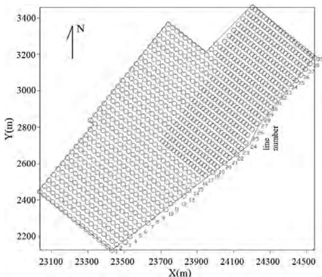
Figure 6. Layout of the survey area showing the 40 m by 10 m grid.
