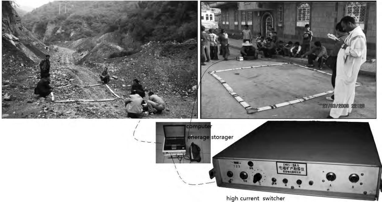
Figure 4. Picture of EMRS-3 system setup during field surveys.
