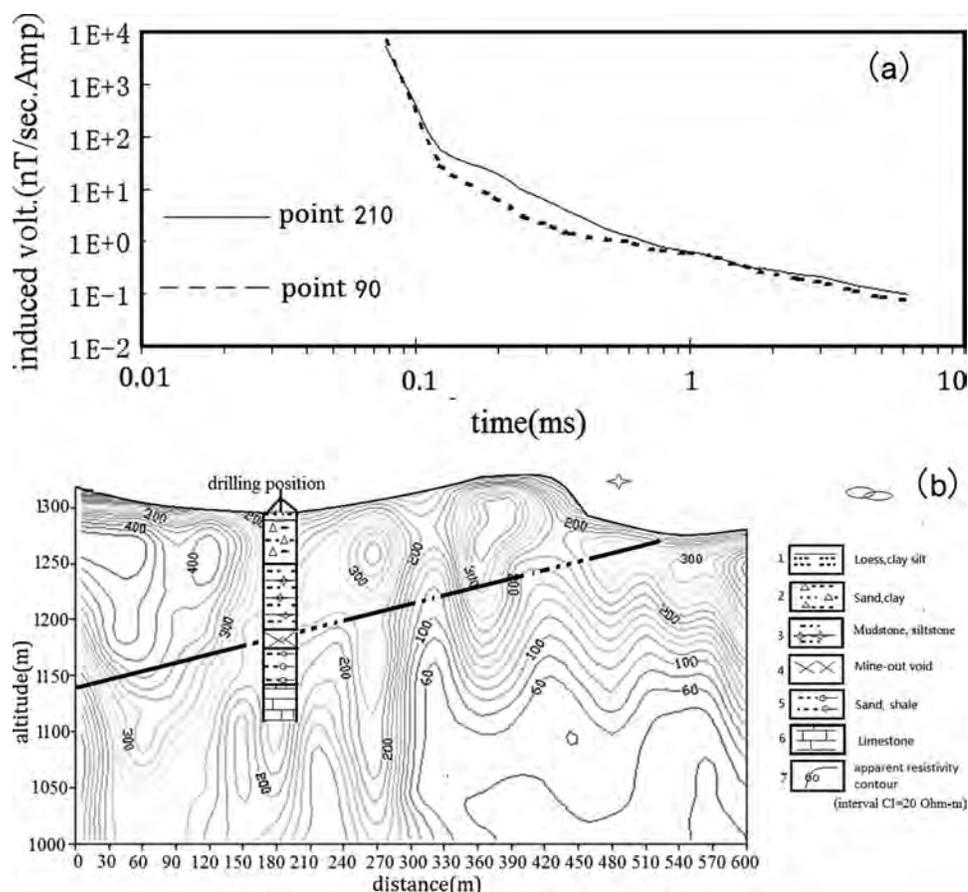
**Figure 8.** Survey result of line 10. a) Decay curve induced voltage at points 210 and 90 along line 10. b) Apparent resistivity contour map and interpreted result for line 10. The drilling result includes the water-filled mined-out space and coal seam. The dashed line connects the water-filled mine cavities at 0 m, 300–330 m, and 400–460 m.
