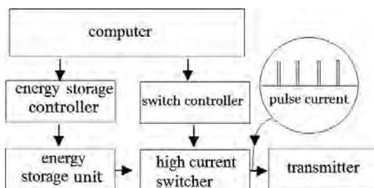
Figure 3. Main system diagram of the EMRS-3 TEM system.
